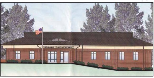
A trussed roof would be added to the structure that previously housed the Highlands ABC Store and brick veneer broken up visually with contrasting brick or rock will be attached to the exterior.
